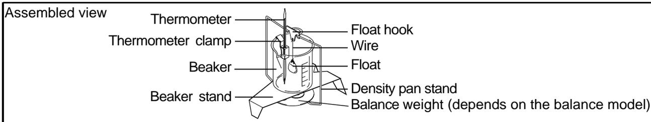
1. For the procedure up to the setting of the beaker stand, refer to the assembly procedure for each balance model described in “5. MEASURING THE DENSITY OF A SOLID”.
