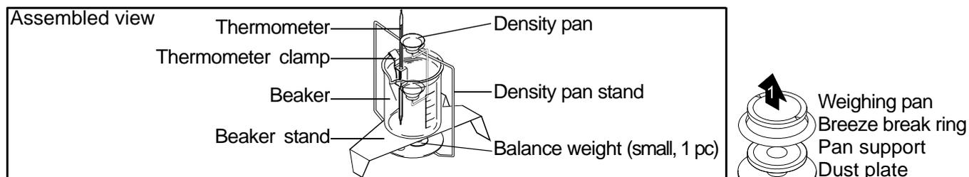
1. Remove the weighing pan, pan support, breeze break ring and dust plate from the balance.
