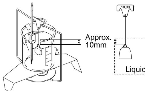
Example: If the measured value (A) is 9.9704 g, the volume of the float (V, printed on the float hook) is 10.00 g/cm<sup>3</sup>, the density of air (d) is 0.001 g/cm<sup>3</sup> and the temperature indicated by the thermometer is 25°C, then the density value is:
